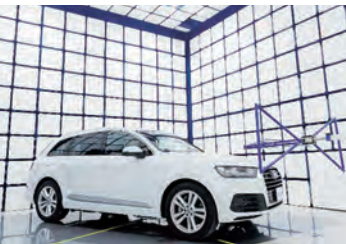
Electromagnetic shielded room We have three electromagnetic shielded rooms in operation, including a large-scale facility capable of accommodating vehicles. These rooms are used for testing and measuring in-vehicle equipment and communications products, and also for conducting various noise and electromagnetic interference (EMI) evaluations.
