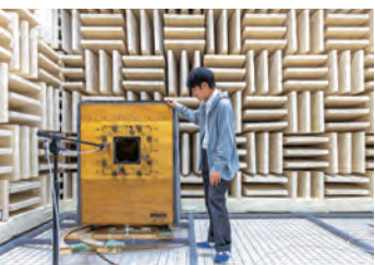
Acoustic anechoic chamber The walls, ceiling, and floors of this facility are fully lined with sound-absorbing material to minimize sound reflections. It is used for the measurement and evaluation of audio equipment.
