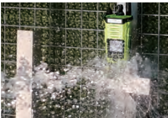
Waterproof testing room This facility recreates environmental conditions such as rain and water spray to evaluate waterproof performance. It verifies whether water infiltration of communications products causes malfunctions, and confirms that the products continue to function normally after testing.
