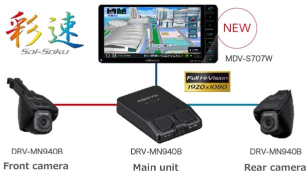
Function for the linkage between a car navigation system and dashcam, which allows a shot video to be checked instantly on a big Saisoku-Navi screen
