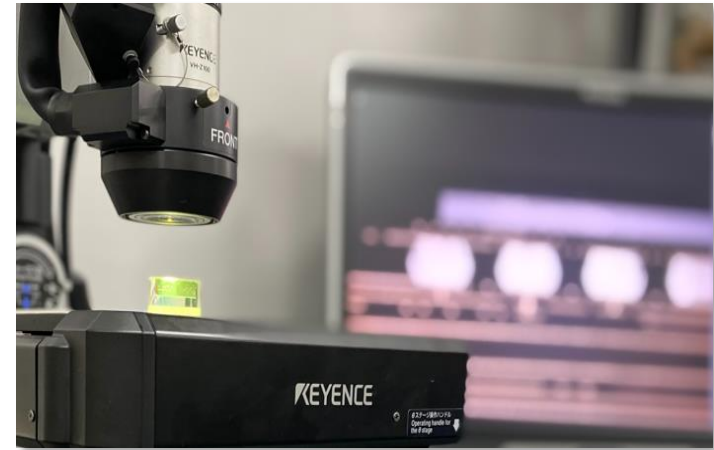
Observation of solder condition by digital microscope
