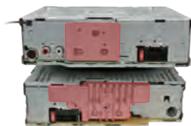
Top : Reduced weight of heat sink by about 50%, and size by about 60% Bottom: Previous model
