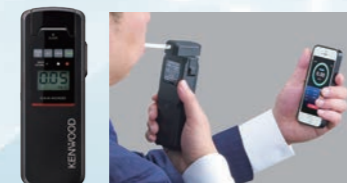
Alcohol detector CAX-AD100 A conceptual image of a communicating alcohol detector that works with a smartphone to send measurement results to the administrator's PC via e-mail
