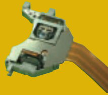
Optical pickup for DVD recorders incorporating a hologram device
