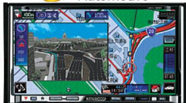
Navigation system integrated with AV for Japanese market (with built-in One-Segment TV tuner)
