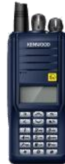
Professional digital radio system “NEXEDGE” compatible with European explosion resistance standards
