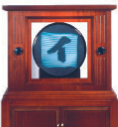
The first image to be projected on a CRT, the Japanese character "イ"
