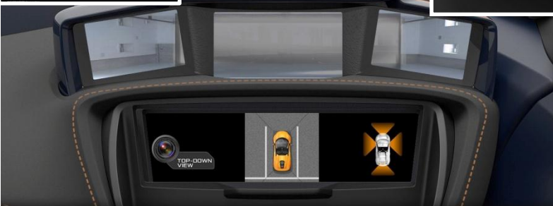
Camera System that provides visibility of 360° around the vehicle with a bird's eye view
